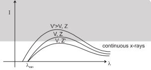
**13.2.1** The minimum wavelength corresponds to the maximum energy of the x-rays which in turn is equal to the maximum kinetic energy eV of the striking electrons thus
