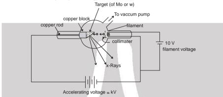
The melting point, specific heat capacity and atomic number of target should be high. When voltage is applied across the filament then filament on being heated emits electrons from it. Now for giving the beam shape of electrons, collimator is used. Now when electron strikes the target then x-rays are produced.
