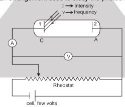
Here the plate (1) is called emitter or cathode and other plate (2) is called collector or anode.
